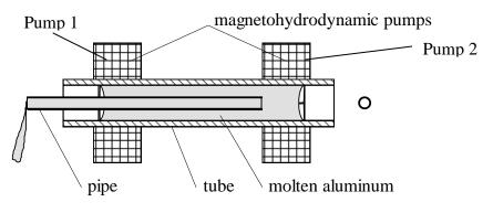
Plating steel pipes
