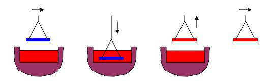
Old process of plating steel rods and pipes with aluminum
