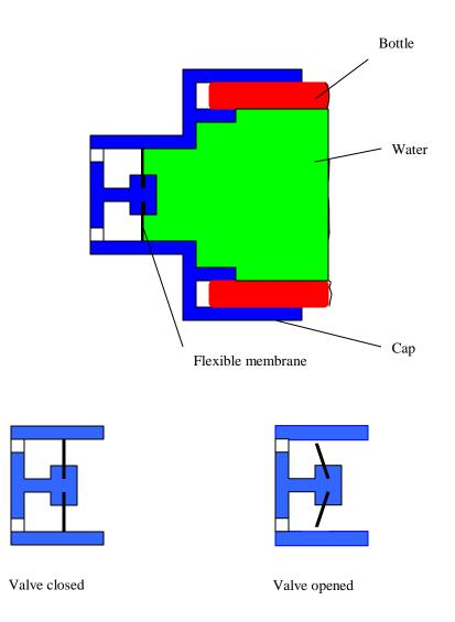
Water bottle cap with a flexible membrane
